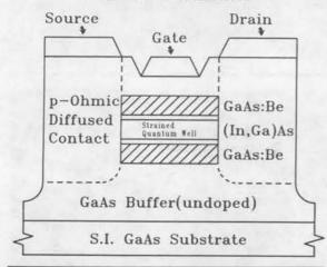
a much smaller effective mass. With decreased mass, the carriers are able to move through the material at greater velocity. Speedier movement of charge carriers leads ultimately to faster devices.
